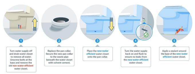
Replacement of a sitting WC will take about 3 hours for each water closet. The sealant will take about 2 hours to dry after application before you can use the new water efficient WC.
