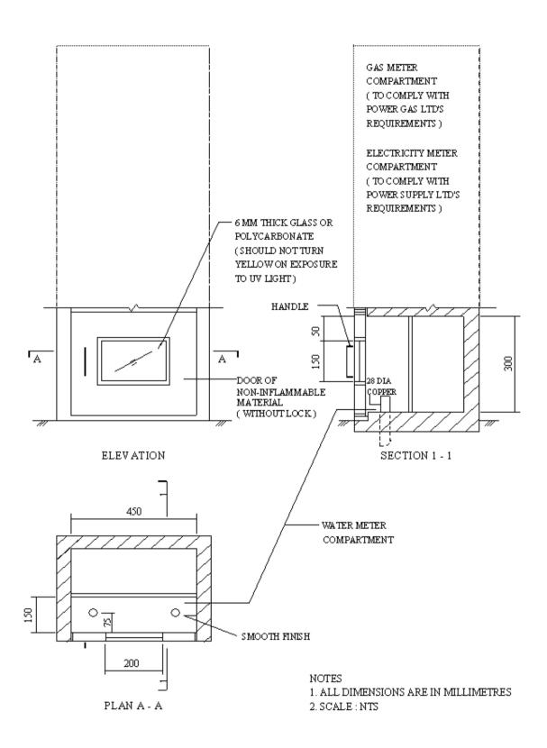
Figure 2 : Standard Water Meter Compartment at Gate Pillar (for Landed Properties)
