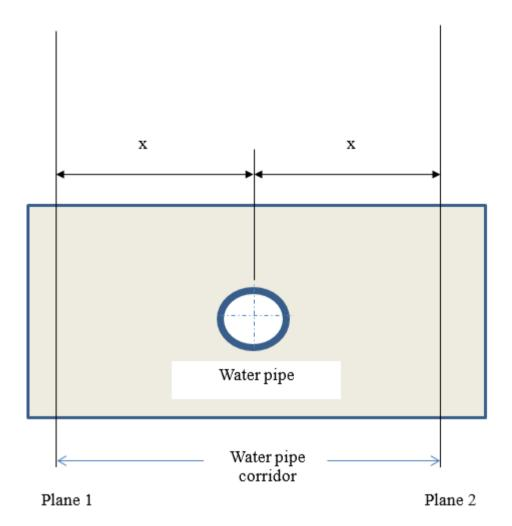
Where "X" is the distance of each of Plane 1 and Plane 2 from the centreline of the water pipe and is —
