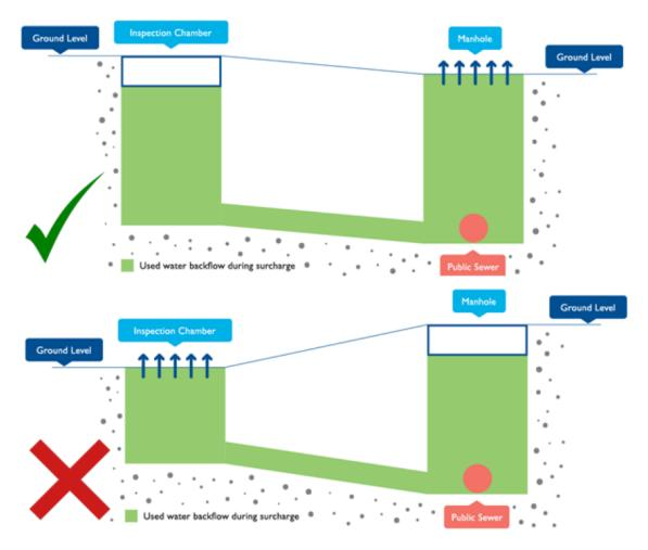
The floor level of the development and the levels of the sanitary appliances, floor traps and inspection chambers should be constructed at levels higher than the manhole to which it is connect to.
