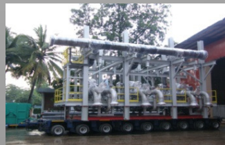
Feed Pump Unit
