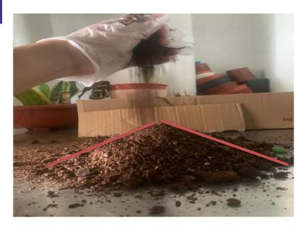
Challenging the 1:3 slope requirements, would potentially compromise the slope stability.
