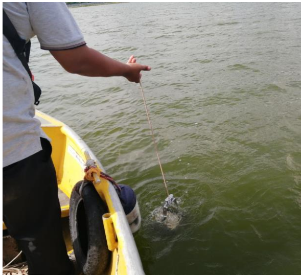
1. Collection of reservoir sediments using Ekman Grab Sampler
