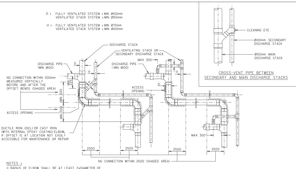
I) RADIUS OF ELBOW SHALL BE AT LEAST 2xDIAMETER OF DISCHARGE STACK. THE ELBOW SHALL BE SECURELY HELD AND BOLTED TO THE BUILDING.
