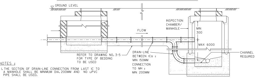
2. THE DRAIN-LINE CONNECTION TO IC/MH SHALL COMPLY WITH REQUIREMENTS IN TABLE BELOW
