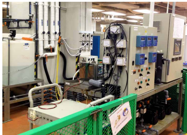
Fig.1: Setup of a laboratory-scale Reverse Electrodeionization (RED)/driven Reverse Electrodeionization (dRED) stack during the pilot study
