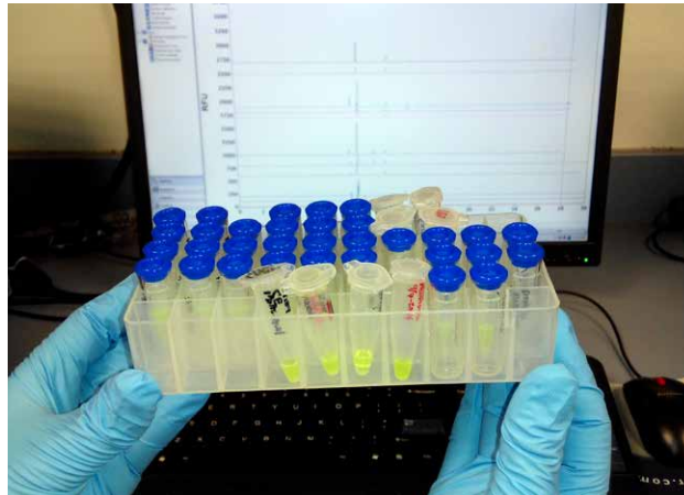
Fig. 2: Samples of extracted endotoxins labelled by fluorescent dye
