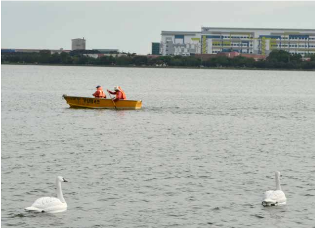
Fig. 1: NUSwan robots performing water quality profiling in Pandan Reservoir
