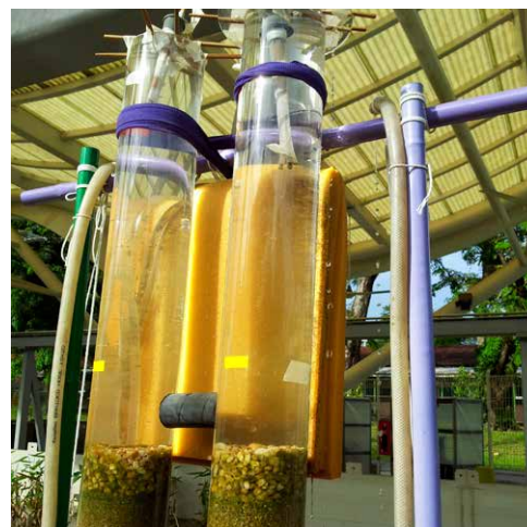
Fig. 2: Column experiments determine the hydraulic conductivity of the designed wetland
