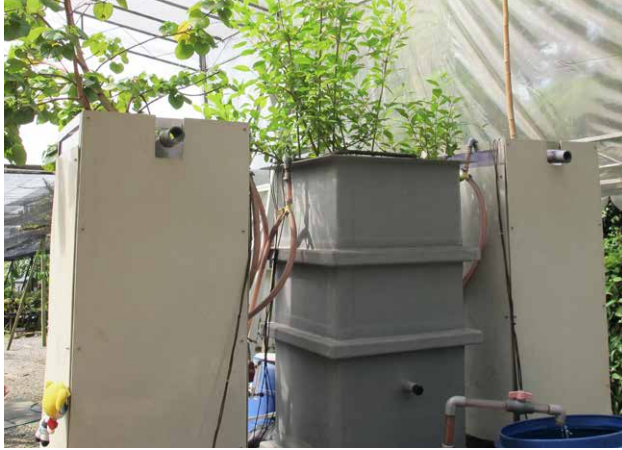
Fig. 1: Pilot-scale bioretention unit to assess the impact of filter media depth and plants on effluent water quality
