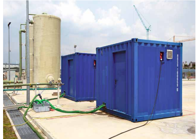
Fig. 2: Pilot plant to test the membranes under actual ultrafiltration operational conditions
