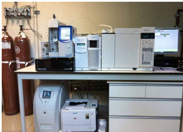
Fig. 1: Set-up of the Purge & Trap — Gas Chromatography Mass Spectrometer (P&T-GCMS) system in Chestnut Avenue Waterworks
