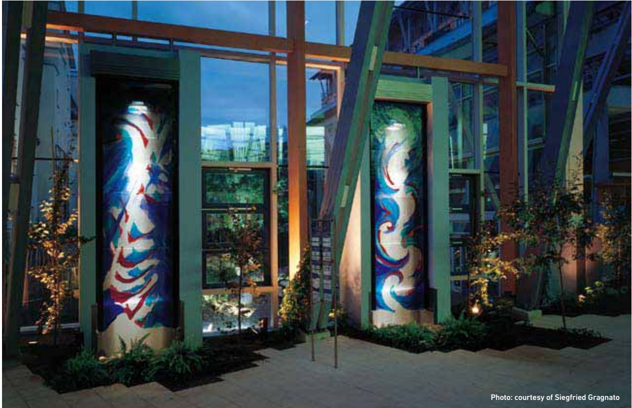
Figure 6.4.5 (Top) Exterior vents supply the water wall with fresh air which is drawn down the falling water and blown out at a wind speed of 3 metres per second. This system helps to regulate the microclimate by cooling the building in summer and warming it in winter, as well as improving air quality over a total volume of 15,000 m 3 in the glass atriums. (Bottom) Cross-sectional view of the water wall circulation system.
