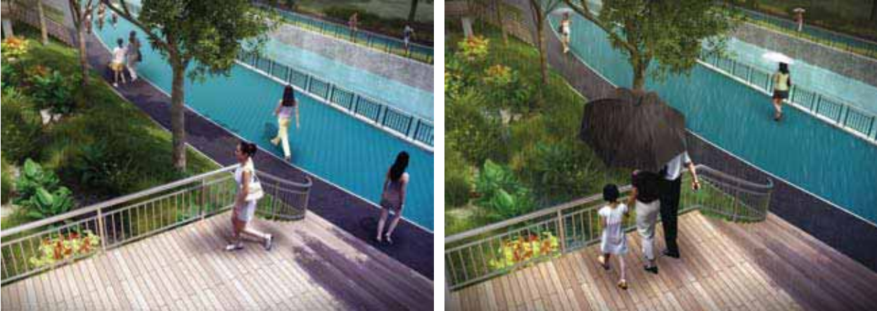
Figure 6.1.2 Bioretention basin during dry weather (left). During a rain event (right), stormwater is directed into the swale, reducing the velocity and volume of runoff into the drainage system.
