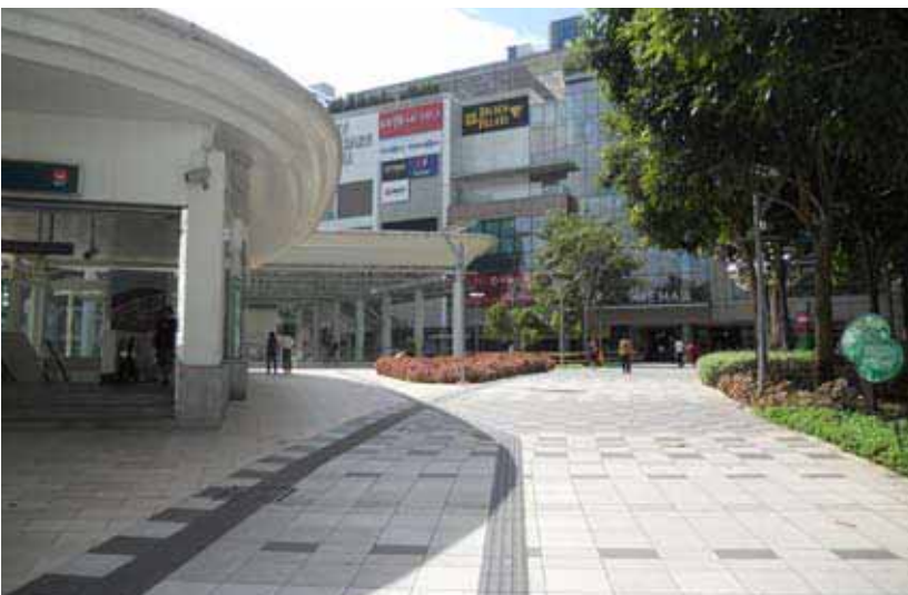
Figure 4.9 The development incorporates an urban park with a sloped access to act as an intermediary area to mitigate the level difference between the road and the platform level of the development, where the entrances are located.
