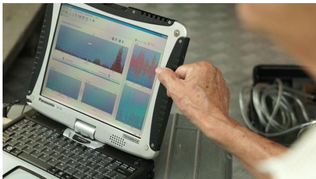
Analysis of noise leak data
