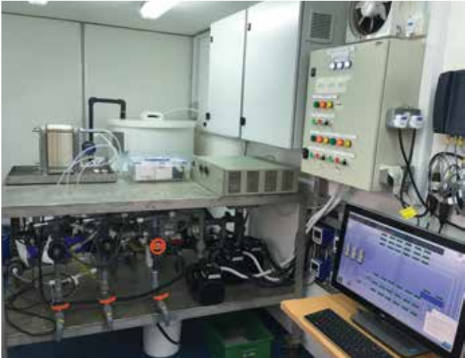
Fig. 3: GE’s RED/dRED pilot system
