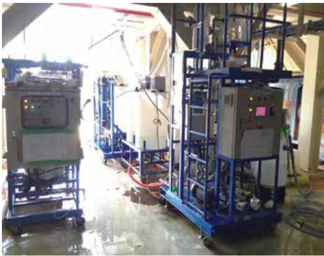
Fig. 4: GlobalFoundries' pilot-scale treatment system for its used water stream
