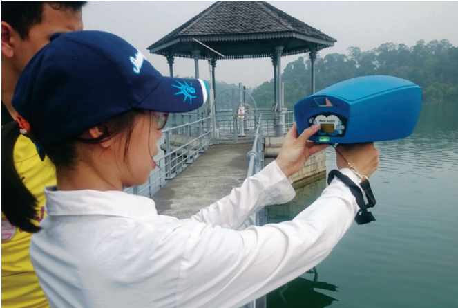
Fig. 1: Testing the WISP-3 hand-held radiometer at a reservoir
