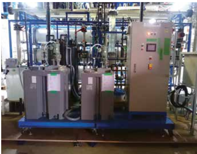
Fig. 5: Pilot-scale ion exchange system used by GlobalFoundries
