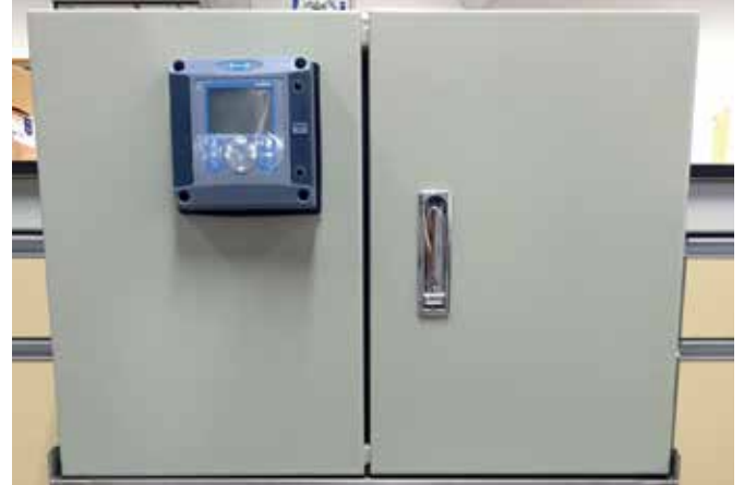
Fig. 2: Compact MES system to be installed at five industrial trade effluent sites
