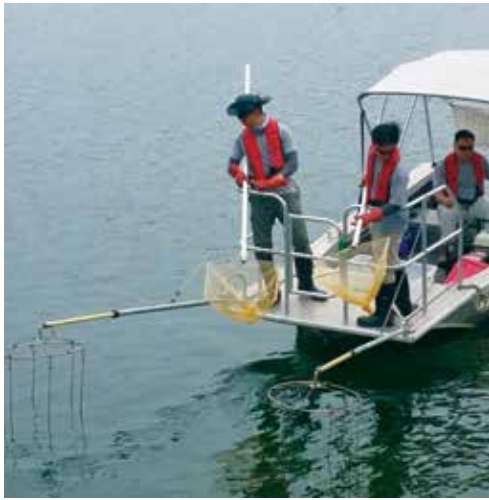
Fig. 1: Researchers conducting electrofishing to sample fishes in the reservoir
