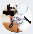
FIG. 6: AMR-enabled inductive meter
