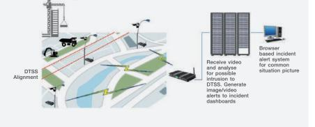
FIG. 1: Concept of operations for surface monitoring along Deep Tunnel Sewerage System (DTSS) alignment
