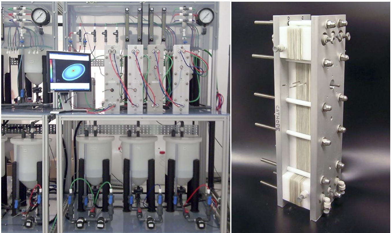
Fig. 1: Laboratory electrodialysis units used to study low-energy desalination solutions
