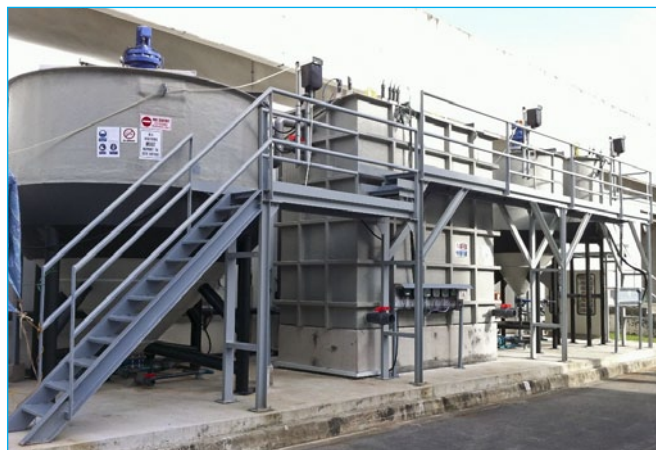
Fig. 2: The 50 m 3 /d pilot plant installed at the Kranji Water Reclamation Plant
