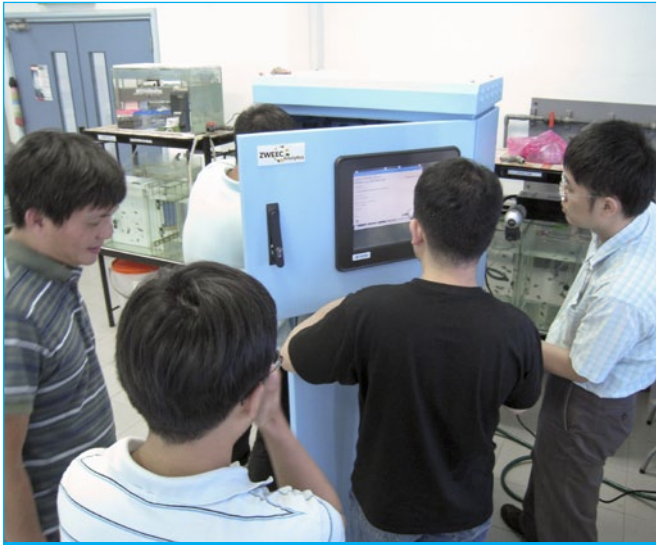
Fig. 1: Researchers install a Fish Activity Monitoring System (FAMS) to monitor raw water quality at the Johor River Waterworks
