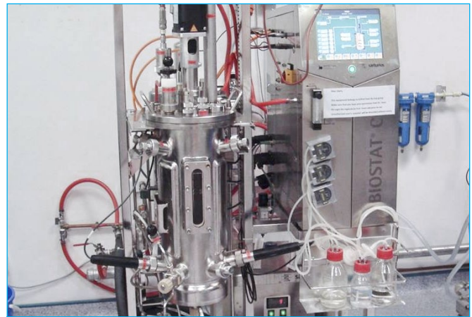
Fig. 2: A bioreactor generates aquaporins ready to be incorporated into a desalination membrane
