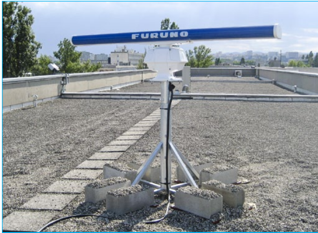
Fig. 1: A typical installation of the LAW system, which provides high-resolution radar scanning over a small geographic region |
