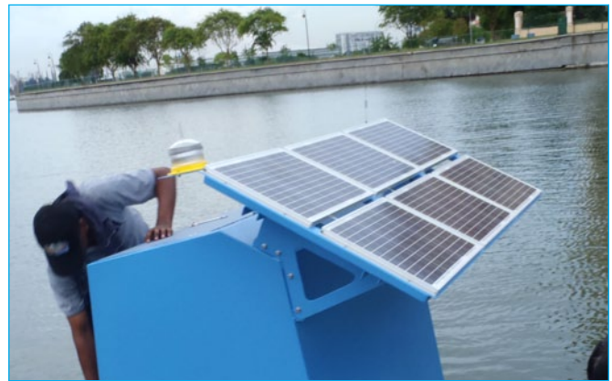
Fig. 2: The moored reservoir monitoring station houses high-resolution instruments for measuring environmental variables
