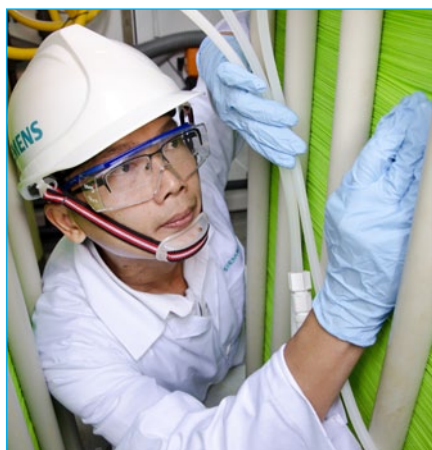
Fig. 1: Inside the new Siemens desalination unit, showing the green ion-exchange membranes
