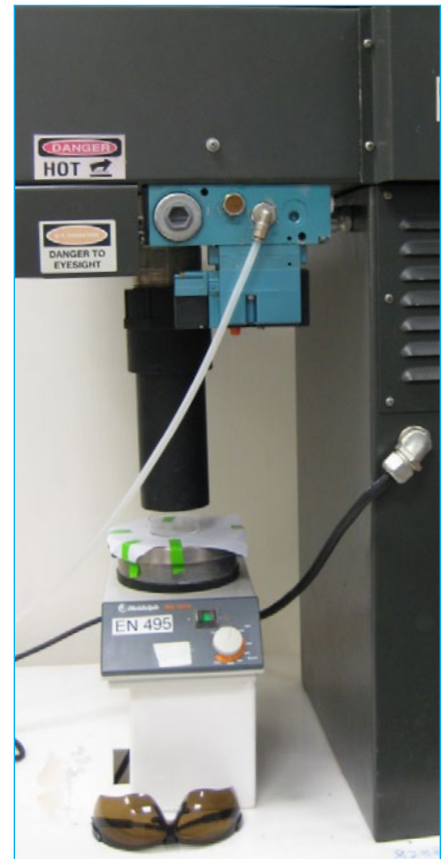
Fig. 1: This laboratory-scale system tests the removal of organic contaminants that are commonly found in urban runoff
