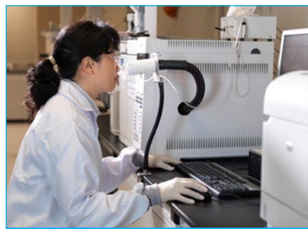
Fig. 1: Using the olfactometry gas chromatograph/mass spectrometer in the PUB laboratory
