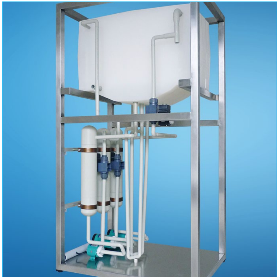
Fig. 1: The memsys desalination system is resistant to damage from oil in water
