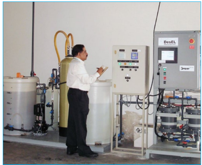
Fig. 2: A pilot plant uses a CDI-based system to recover much more clean water from waste sources than existing treatment plants
