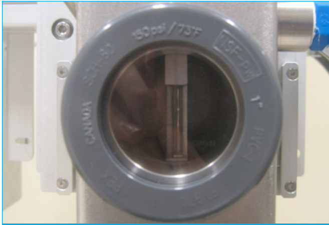
Fig. 1: The laser-based sensor cell of the EventLab networked water quality monitoring system
