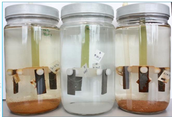
Fig. 1: Untreated seawater reverse osmosis water can have deleterious effects on small metal-strip samples of ductile iron (left), cement-lined (centre) and cast iron (right) pipes
