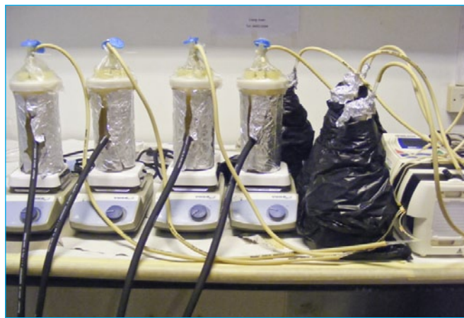
Fig. 2: Biological growth experiments reveal that remineralization of water protects pipes from corrosion but also provides a breeding ground for bacteria
