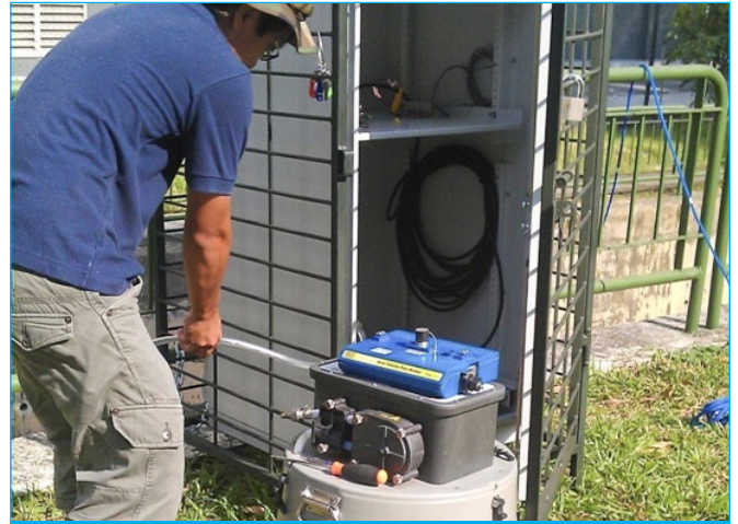
Fig. 2: Automated stormwater sampling devices installed at sites across Singapore are measuring the levels of heavy metal contaminants
