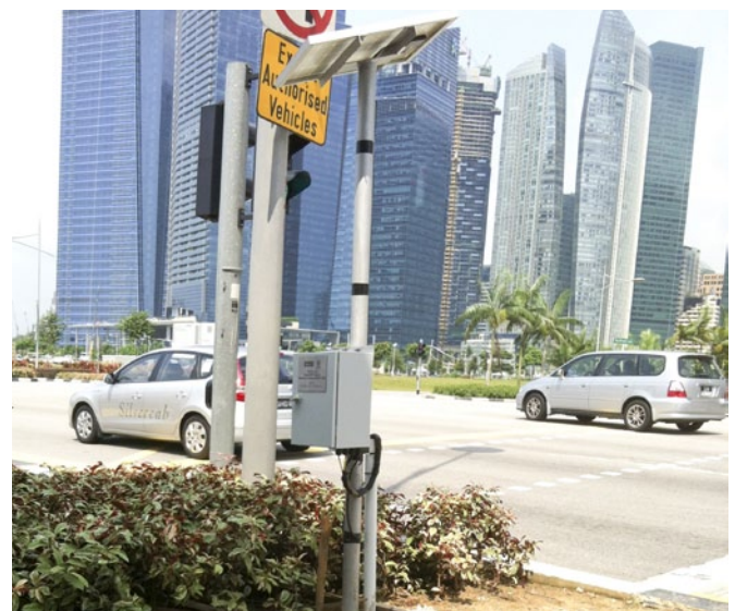
Fig. 2: The new nodes are powered by batteries that are recharged by solar panels and adjacent street lights
